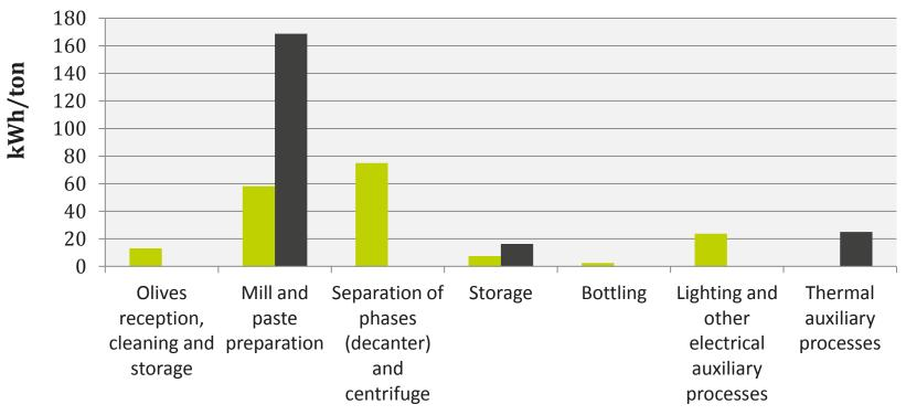
Electrical energy consumption (kWh/ton) Thermal energy consumption (kWh/ton)
